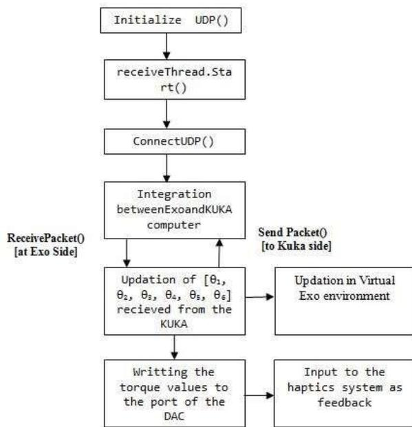
Figure 3. System architecture based on UDP protocol [3]
